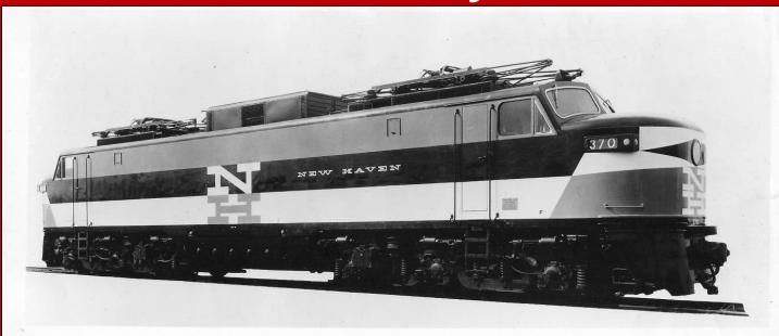
5015730-A Erie Works File G-E Rectifier Locomotive, 174 Ton, 56 1/2 In. Gage, Classification C-C-346/348-6GE752 Motors - 4000 Hp, 11000 Volt AC, 600 Volt DC, Serial No. 31931-31940. Bult for New York, New Haven and Hartford R. R., Req. NH-17100. Oblique View of No. 1 End. A Side.
