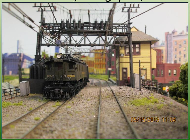
Home Signals mounted on catenary bridge. Note the blades are left-handed.
